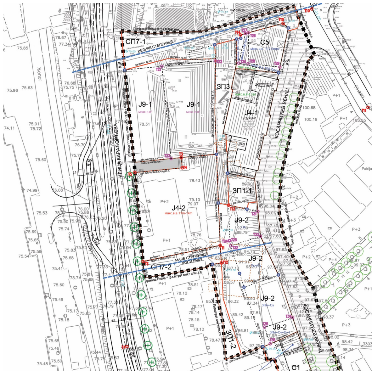
Excerpt from Amendment of the Detailed Regulation Plan for Spatial Unit Kosančićev venac for the block part between the following streets: Karađorđeva street, Velike stepenice and Kosančićev venac, in the City Municipality of Stari grad (“Official Journal of the City of Belgrade”, no. 76/21), Graphic Enclosure 04 “The Regulation and Levelling Plan with the Analytical and Geodetic Marking Elements”
